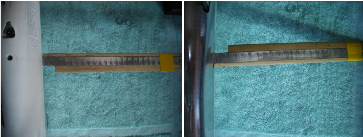
Wood streamlining fitted to the bridle, the metal can be seen and it can be measured.
