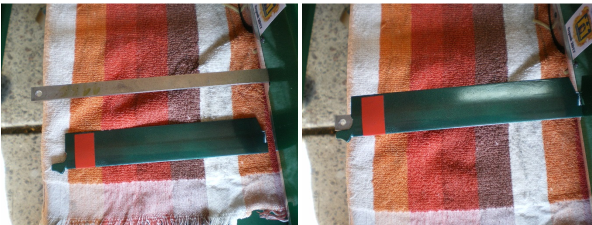
Without the streamlining the metal is clearly visible the streamlining slides over the bridle
